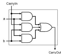
The program should accept three inputs: a, b, CarryIn, and generate one output: CarryOut. As before, check that the keyboard input is 0 or 1. Remember, you are **not** implementing the complete 1-bit adder circuit, only the CarryIn / CarryOut part.
