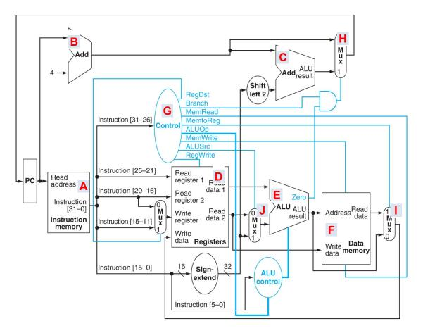
• Refer to the labels **A** through **J** in the datapath diagram above, which components are required during the execution of **lw** instruction? To answer this question, please cross the components from the following table that are not used for executing a **lw** instruction. [0.5 mark]
