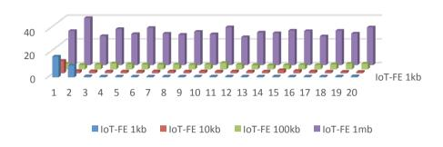
FE to Cloud communication time is significant compared to IoT-FE and FE-FE communication times (as expected).
